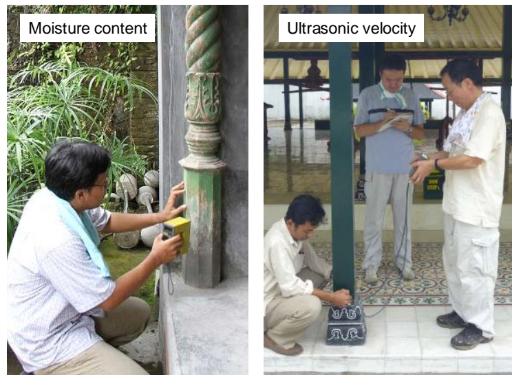
Figure 3. Measurement of moisture content and ultrasonic velocity
