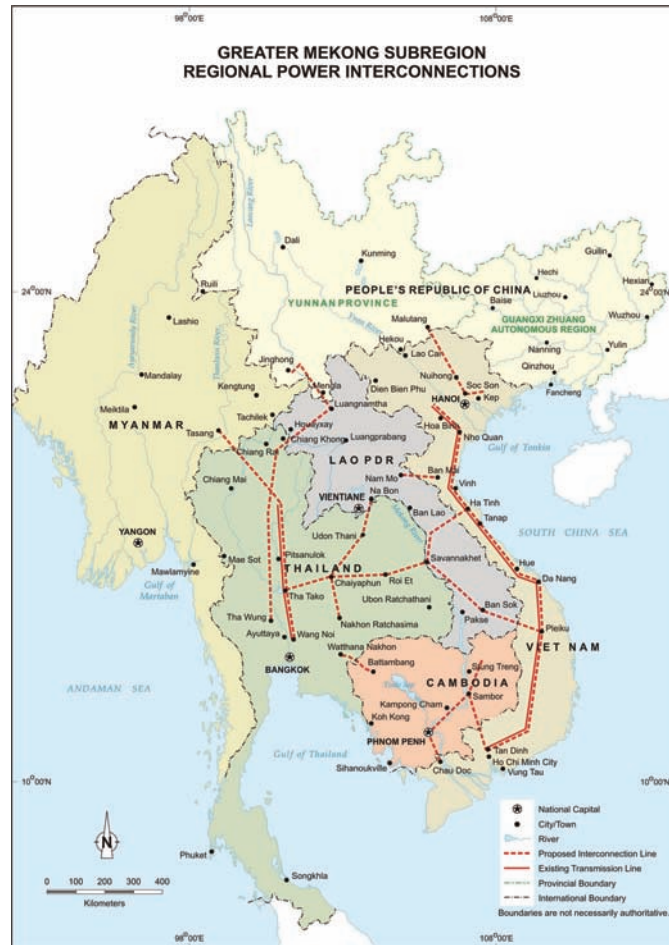
Figure 2.2 Regional power interconnections in GMS
