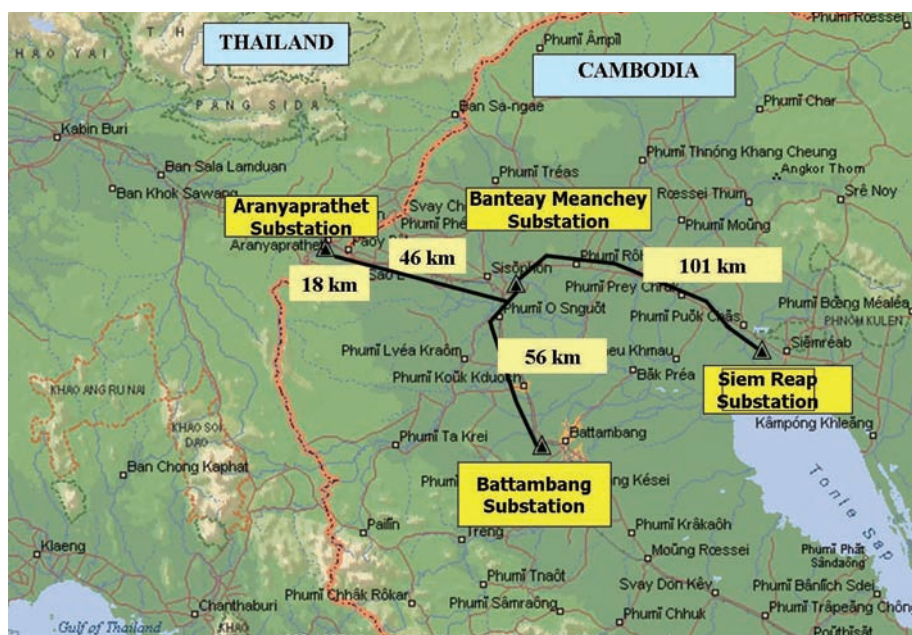
Figure 2.9. Thai-Cambodia power interconnection
